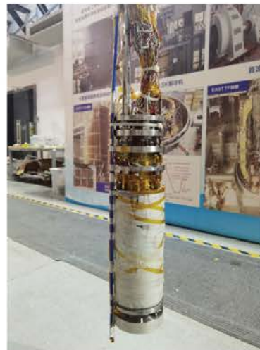
Fig.2 Photo of fabricated 20-T magnet before liquid-helium test.
